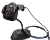
LS 2208 Single Line Laser with Stand 100 Scan/sec Auto/Manual Trigger
